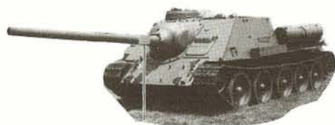
SU-100 — the improved version of the SU-85 mounted a 100mm gun, L/54.
